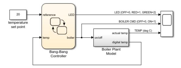
The example consists of a Stateflow chart and a Simulink® subsystem. The Bang-Bang Controller chart compares the current boiler temperature to a reference set point and determines whether to turn on the boiler. The Boiler Plant Model subsystem models the dynamics inside the boiler, increasing or decreasing its temperature according to the status of the controller. The boiler temperature then goes back into the controller chart for the next step in the simulation.
