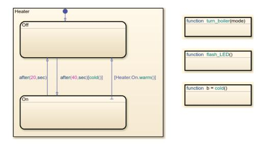
The actions guarding the transitions between the On and Off substates define the behavior of the bang-bang controller.
