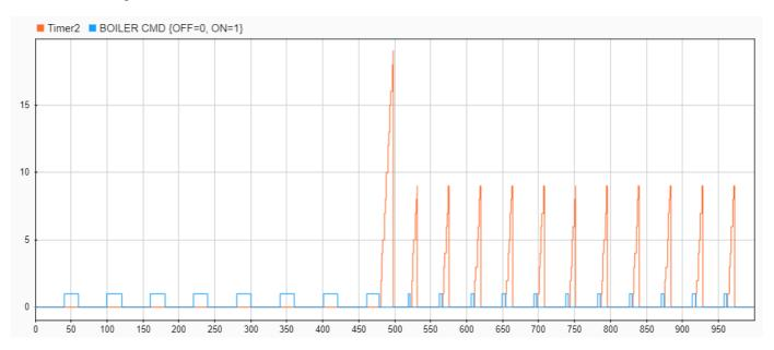
The shorter cycle and longer cooling time are a consequence of the substate hierarchy inside the On state. When the boiler reaches the reference temperature for the first time, the transition from HIGH to NORM keeps the controller on for an extra time step, resulting in a warmer-than-normal boiler. In
